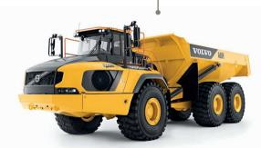
Built on the proven Volvo technology of articulated steering, all-wheel drive and differential locks, the Volvo A60H has evolved to be bigger and bolder!
